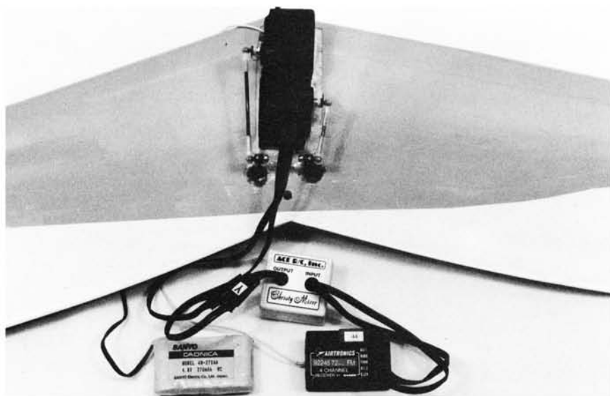
View of the wing's underside shows the mounted servos hooked to radio gear (above) that consists of a 250 mAh flat battery pack, ACE Christy Mixer, and Airtronics 92245 receiver. The radio gear mounts on a ply plate (below) that is then fastened inside the body/fuselage with RTV silicone. The pattern for the ply plate was made from the trial and error fit of a piece of cardboard shown.
